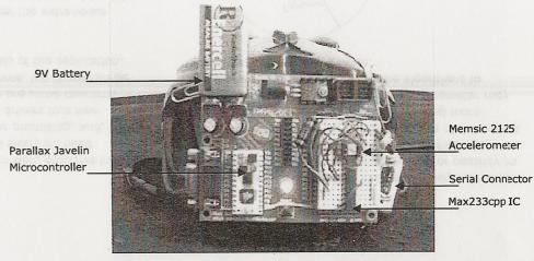
**figure 3.** The interface board as installed on the back of a bicycle helmet.
