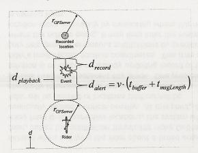
**Figure 5.** Decomposition of the distance at which a recorded notification should be played back to the rider, with respect to the location at which the recording began.
