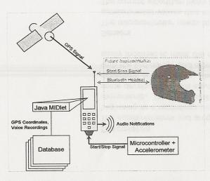
**figure 2.** System diagram for both the current and future implementation of the location-based notification system.
