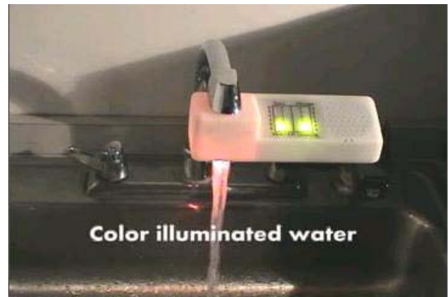
Figure 5. Random patterns in color illuminated water act as reinforcers to reward consistent water-saving behavior. Reinforcers also help to keep users interested.
